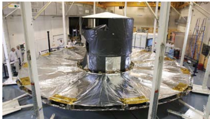
The spacecraft after deployment of the sunshield in the cleanroom
