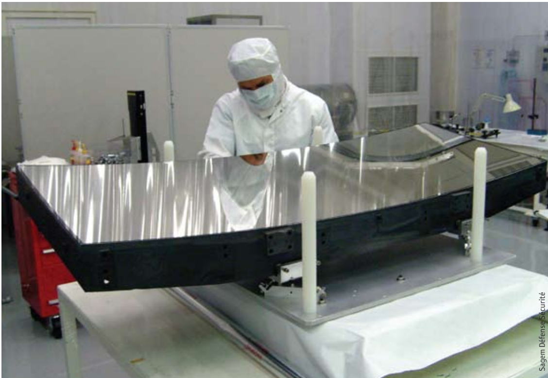
Final check of one of Gaia's primary mirrors
