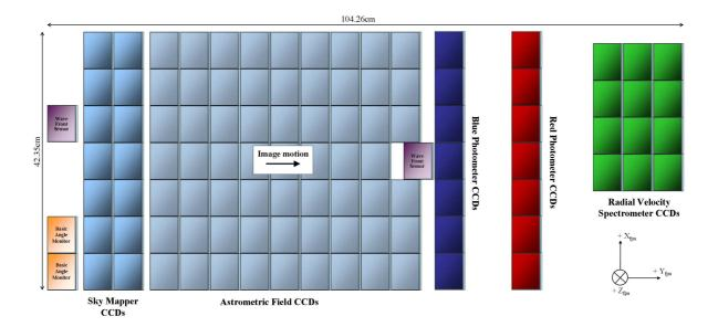
The Gaia focal plane. The viewing directions of both telescopes are superimposed on this common focal plane which features 7 CCD rows, 17 CCD strips, and 106 large-format CCDs, each with 4500 TDI lines, 1966 pixel columns, and pixels of size  $10~\mu m$  along scan  $\times$   $30~\mu m$  across scan (59 mas  $\times$  177 mas). Star images cross the focal plane in the direction indicated by the arrow. Figure courtesy of ESA - A. Short.
