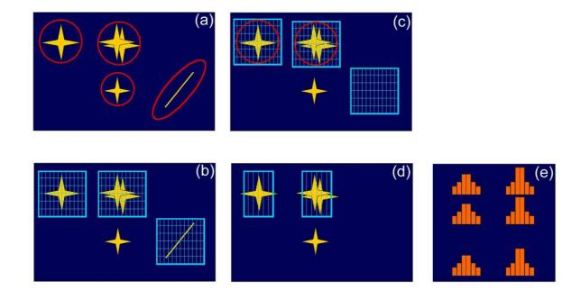
The on-board data handling consists of a sequence of operations starting with (a) object detection, (b) first selection, (c) actual observation in the next CCD strip and confirmation, (d) final selection, (e) observation in the following CCD strips, post-processing with packetisation, and compression for subsequent downloading.
