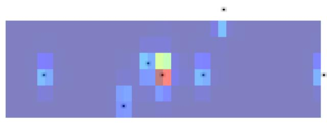
saves the read-out from the CCD in a window around the star
