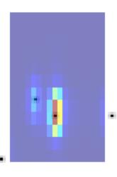
Detection data used to read out from the Astrometric Field CCDs
