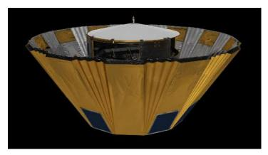
Figure 1 – The unfolding of Gaia's sunshield with its solar panels on the back.
